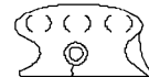
ONE CRACK EXTENDING ABOVE SET SCREW NOT PERMISSIBLE. ONE CRACK BELOW SET SCREW PERMISSIBLE.
